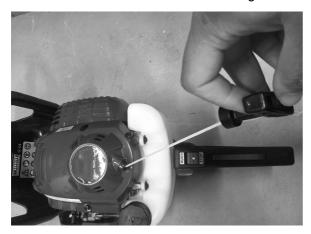
Push and hold throttle trigger lockout (1) and then push the throttle trigger (2).
